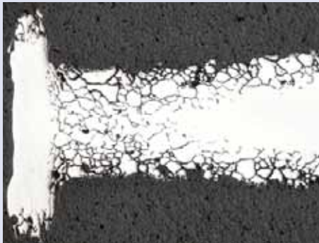
Micro section showing a nice example of intergranular corrosion in a bolt made of 4307. The cause of the sensitization is not the C from the steel itself, but rather the use of oil. A subsequent heating process has released the carbon, which in turn has diffused into the steel. Thereafter, the Cr has been bound as carbides, and a subsequent pickling process caused the sensitization to turn into IG.
