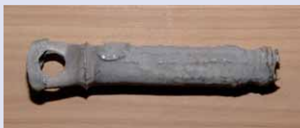
4301 stainless steel bolt suffering from severe general corrosion after having spent a number of months in a nitric acid-hydrofluoric acid pickle bath. Please note that the loss of metal is quite uniform and quite large while no penetration has occurred yet.
