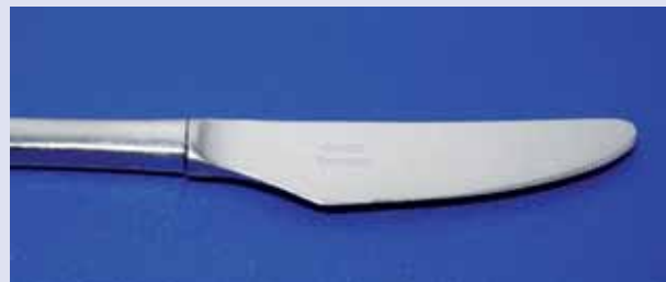
The ideal combination in between hardness and formability. The blade of this Gense knife has been manufactured from the martensitic 4057, while the handle has been made of the softer, but more corrosion resistant 4301.
