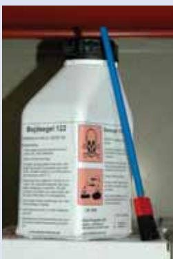
Left: Steel-Tech "Pickle Gel 122", a nitric acid + hydrofluoric acid based paste, useful for nor-mal stainless steel. Applied by using a special brush. Right: Using pickling paste on a weld on the inside of a 4436 steel pipe.
