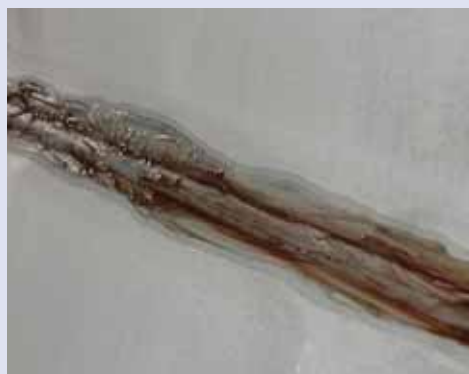
Left: Steel-Tech "Pickle Gel 122", a nitric acid + hydrofluoric acid based paste, useful for nor-mal stainless steel. Applied by using a special brush. Right: Using pickling paste on a weld on the inside of a 4436 steel pipe.
