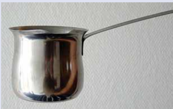
Ferritic stainless steels are very useful for manufacturing thin-walled specimens without too much welding or bending. This Syrian made kitchen utensil has been made of 4016 (AISI 430), a very common steel within catering and a perfect example that it is actually possible to perform deep-drawing in ferritic stainless steel.
