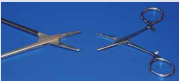
Surgical instruments, both made of martensitic stainless steel. Their mechanical strength is impressive, whereas the corrosion resistance is low.
