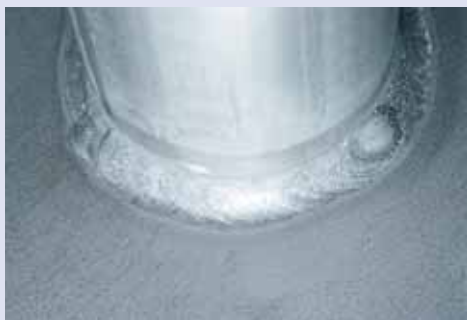
Pickled weld on a 4404 specimen. Please note that the specimen appears slightly mat – almost like after a glass blasting. This is because of the increased surface roughness due to the etching of the steel.
